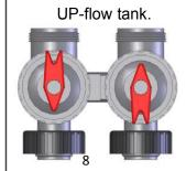
Bypass Position UP-flow tank.
